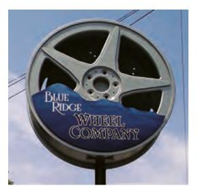
6-ft.-tall, 30-in.-thick, two-sided wheel with slotted and cross-drilled brake-rotor to prevent view-through. All HDU with steel mounting assembly to tie into existing post, and a lot of airbrush work to add detail.
