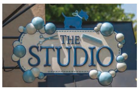
3-ft.-wide HDU sign with carved HDU soap bubbles. Integral aluminum structure has a custom bracket with down lights. Three LED fixtures are integrated into bottom to light walkway and entrance. Photo by Dragon Ridge Photography
